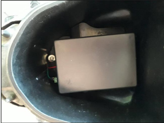
Fig. 4. The installation of the proposed device on a motorcycle (under seat).
